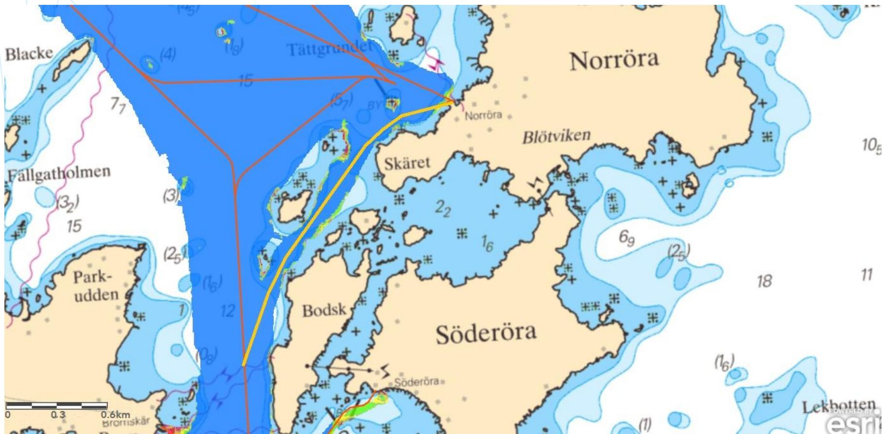
Suggested route adjustment Norröra and Söderöra which results in a better weather shelter and a time- and fuel saving route.
