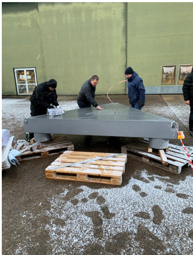
Figure 6 New calibration target near Frederikshavn before placing on the sea floor.
