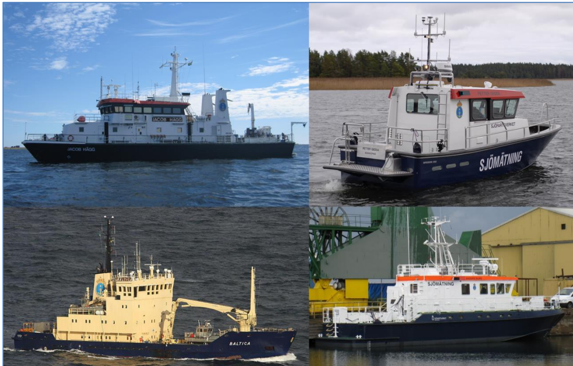
Figure 3- SMA Survey vessels equipped with multibeam. To the left the two survey vessels Jacob Hägg and Baltica where surveying is performed 24 hours per day and 7 days per week, weather permitted.
