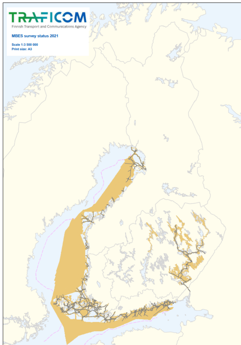
Fig.2. Hydrographic re-survey coverage at the end of 2021 surveyed according to IHO S-44 and FSIS-44 standards.
