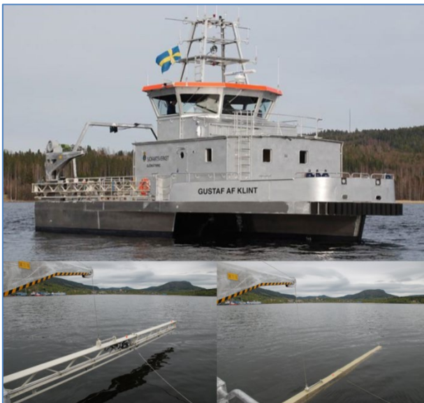
Figure 4 Bar sweeping survey vessel Gustaf af Klint. The bar is transverse across the stern and submerged into the water.
