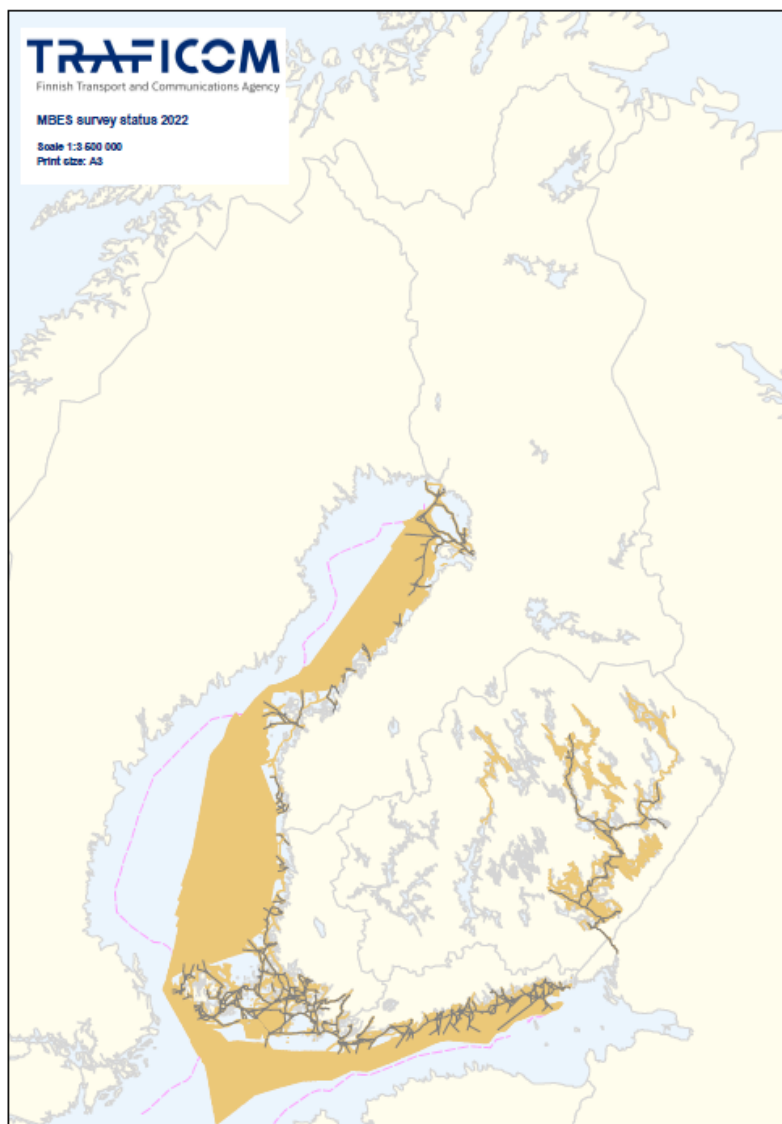
Fig.2. Hydrographic re-survey coverage at the end of 2022 surveyed according to IHO S-44 and FSIS-44 standards.
