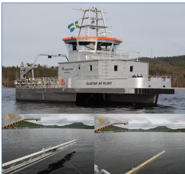
Figure 4 Bar sweeping survey vessel Gustaf af Klint. The bar is transverse across the stern and is here submerged into the water.
