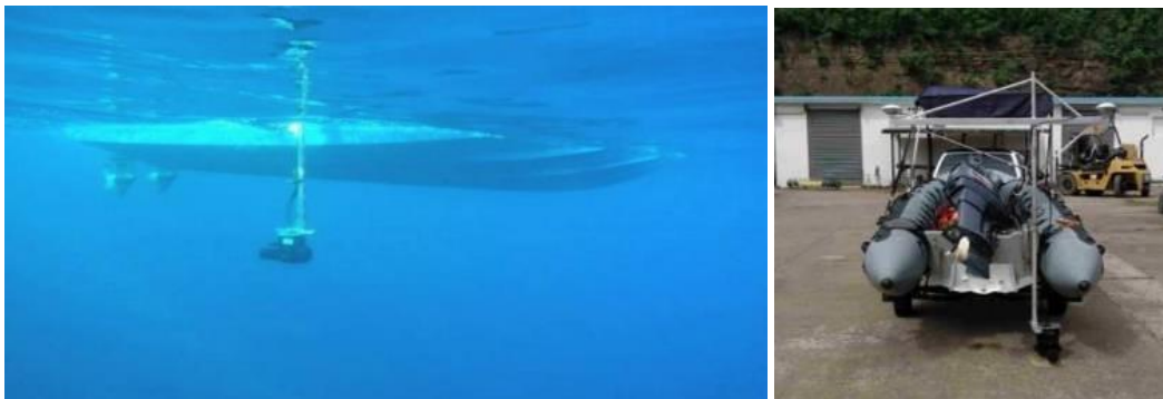
Fig. 1 – MBES Norbit iWBMSH integrated to Shom's deployable hydrographic system
