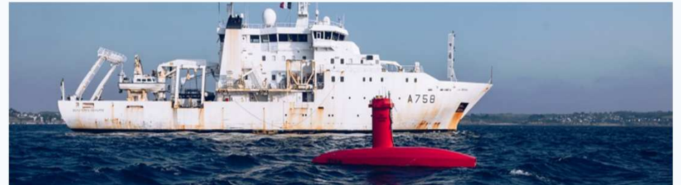
Experiment of USV DriX deployed from BHO Beautemps-Beaupré
