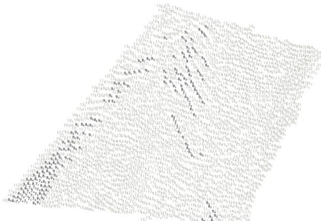
Figure 4: Thames Estuary multibeam survey is then turned into a sounding selection by a trained cartographer (in this case at 1:50000) and the data is heavily filtered to achieve this
