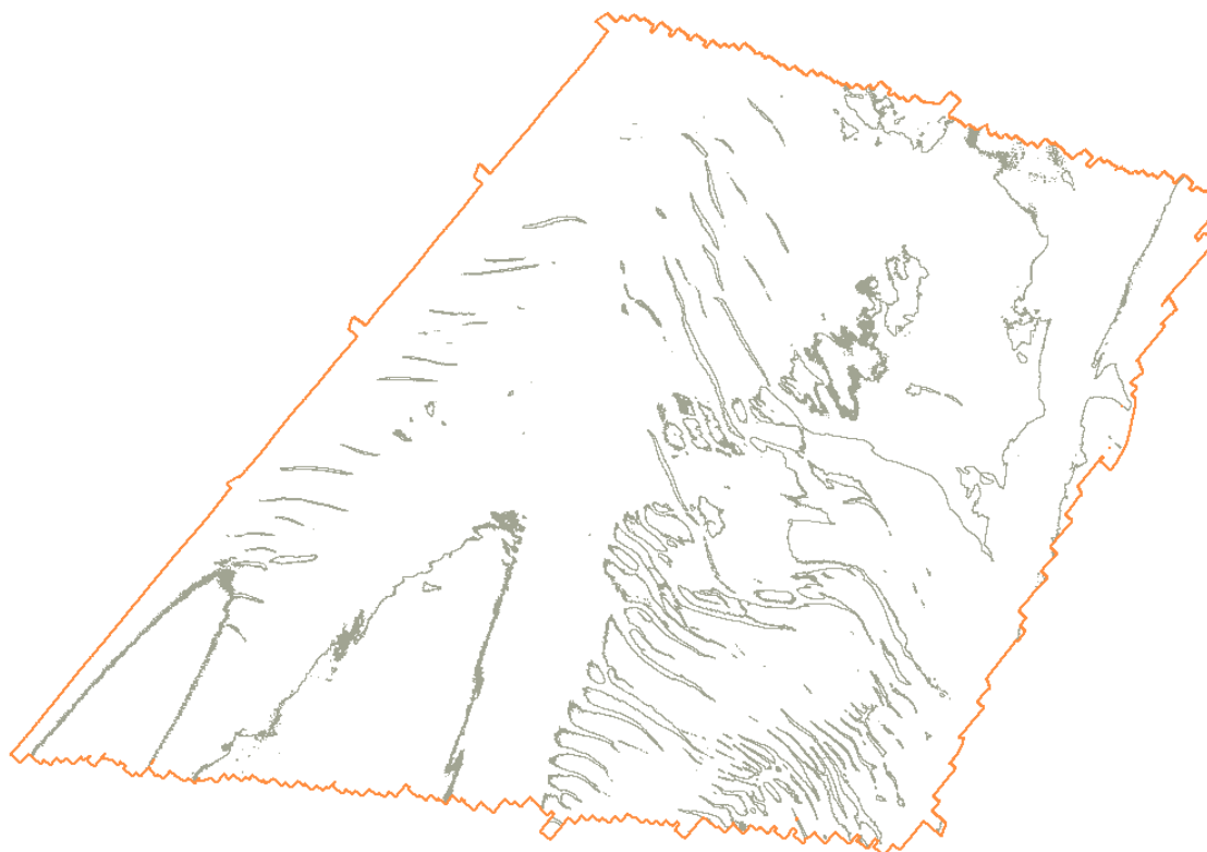
Figure 5: The sounding selection is then turned into depth contouring at standard interval (further filtering of data).
