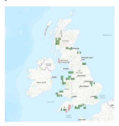
Rather than produce additional HD ENCs, UK is focussing on including areas of supplementary contouring (at 1m or 0.5m intervals) within the gridded ENCs. These are treated on a case by case basis, but generally focus on port approaches and confined channels to provide better safety contour representation of usable water.
