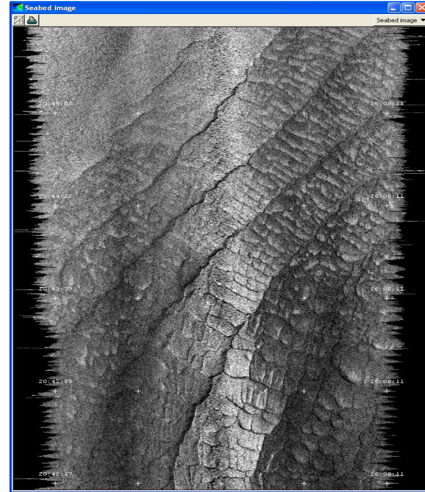
Sandwaves, 90 - 100m depth, 300 kHz / 70us
