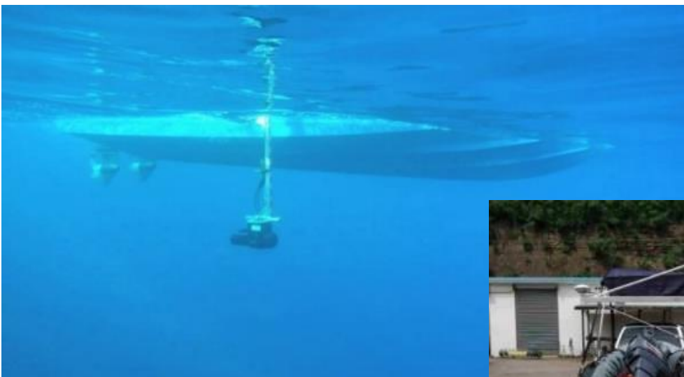
MBES Norbit iWBMSH integrated to Shom's deployable hydrographic system
