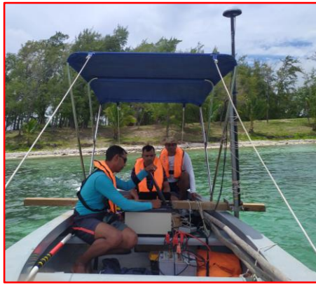
Figure 4: Singlebeam Survey at Belle Mare
