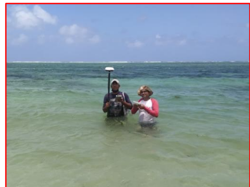
Figure 6: Pole Sounding at Surinam
