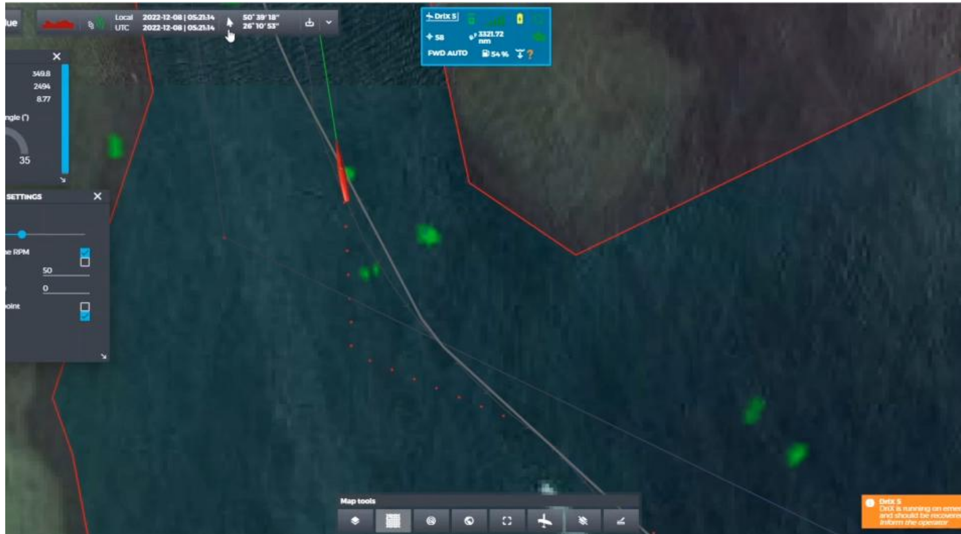
Dec 8, 2022 - Autonomous entry and collision avoidance in Mina Salman, Barhein. (Speed 10 knots, video speed x20). CPA setting 100 yards
