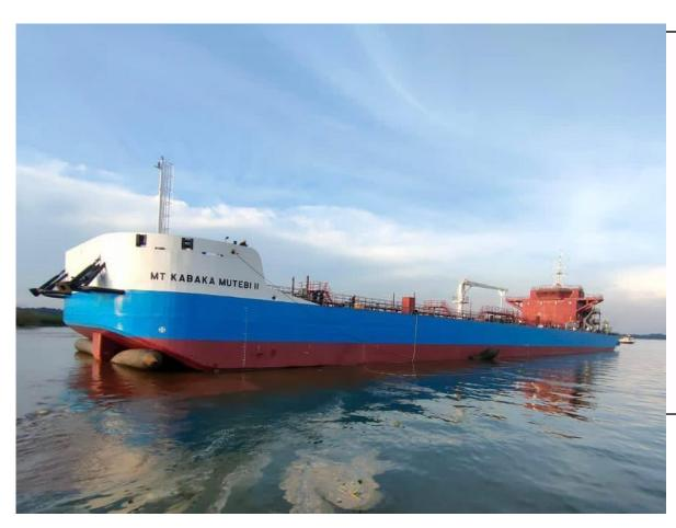
The oil tanker has a cargo capacity of up to 4.4 million litres of petroleum cargo with a deadweight of 3,687 tonnes measuring 118m by 23m and a draft of 2.5m
