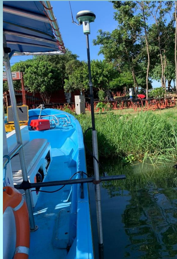
Single Beam survey complemented by terrestrial bathymetry
