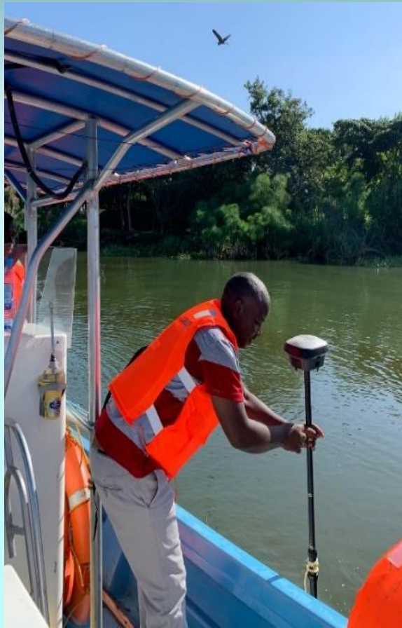
Single Beam survey complemented by terrestrial bathymetry
