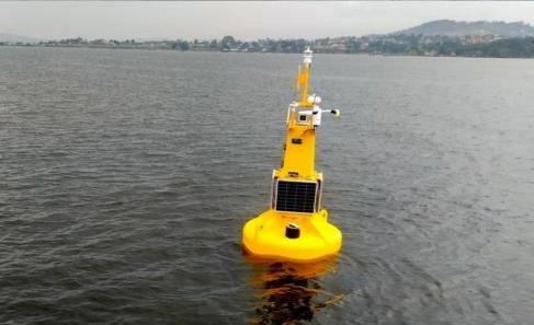
The buoys are to provide real time recording of the prevailing weather conditions on the lake.
