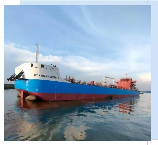
They have two oil tanker with each has carrying capacity of up to 4.4 million litres of petroleum cargo with a deadweight of 3,687 tonnes measuring 118m by 23m and a draft of 2.5m
