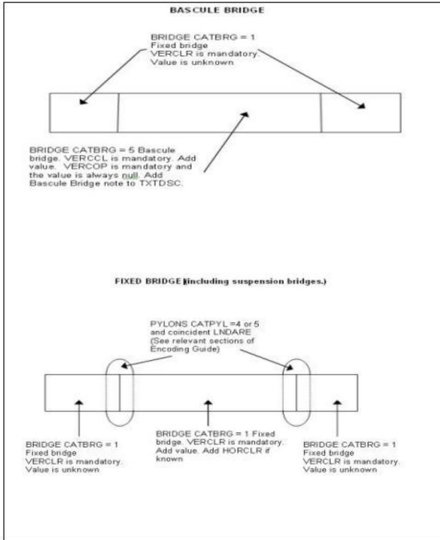
Bridge Encoding Diagram
