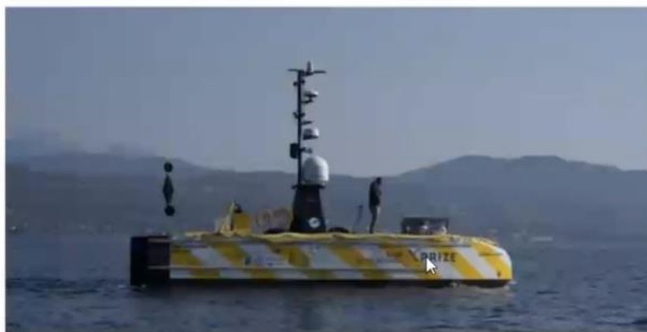
Figure 2. USV SEA-KIT 'Maxlimer' during the preparation to the final survey, Kalamata, Greece: the surface part of the mapping devices set used in Round 2 of Shell Ocean Discovery XPRIZE (Photography by XPRIZE).
