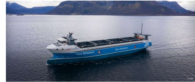
MV Yara Birkeland, first autonomous and 100% electric container ship
