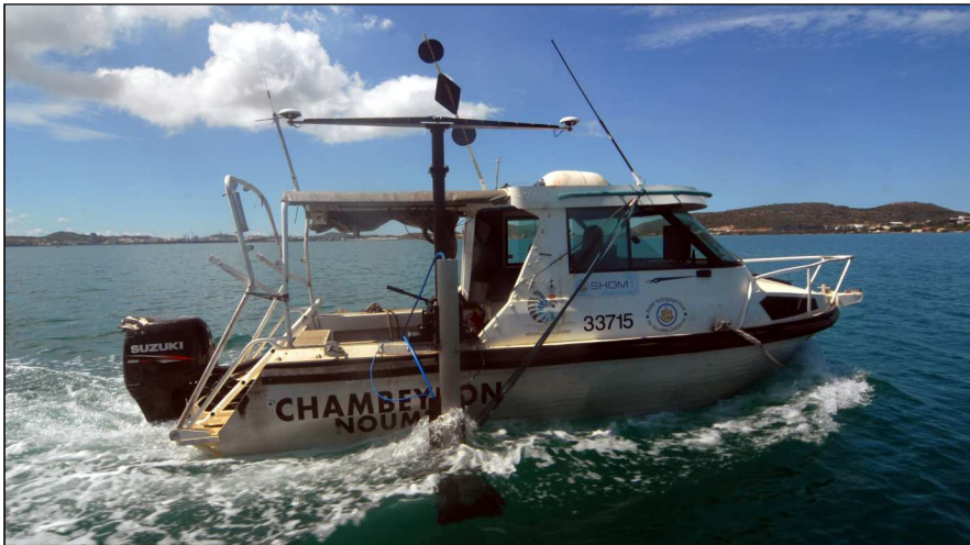
Fig.19 & 20: HSL Chambeyron with multibeam echosounder.
