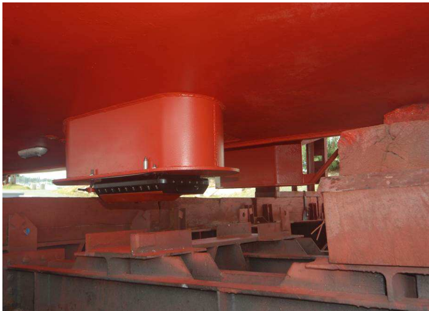
Fig.21: Multibeam echosounder installed on Buoy-Laying Vessel Louis Hénin
