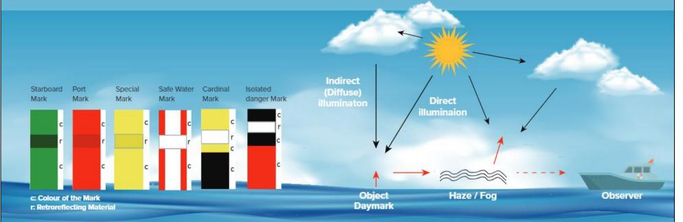
AtoNs can be equipped with retroreflective material, so the mariner can detect the position and colour at night by use of a searchlight
