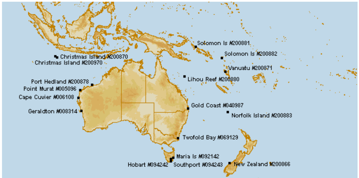
Fig. 2: Additional ATWS radar gauges (17 sites) that used in conjunction with the permanent tide gauge network for monitoring tsunamis in the Australian region.
