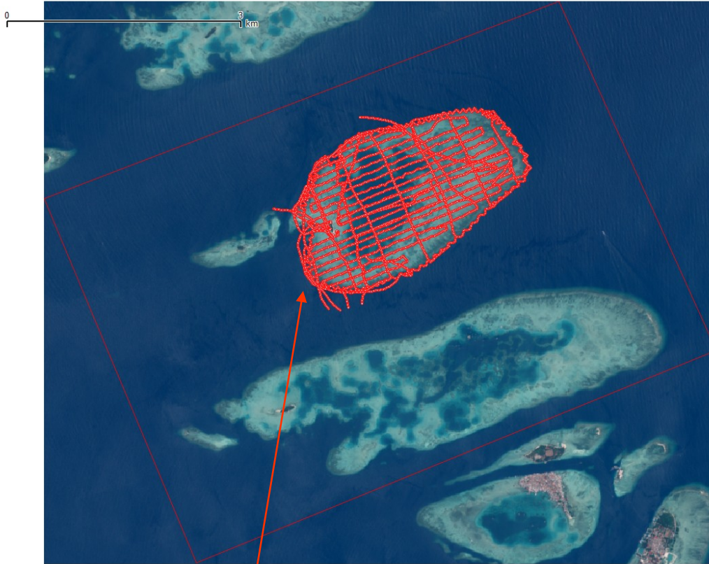
Survey data, single beam, Gosong Congkak Source: Hydrography Laboratory ITB
