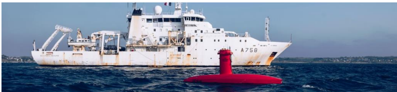
Fig. 26 - Experiment of USV DriX deployed from BHO Beautemps-Beaupré (Source: iXblue, 2020)
