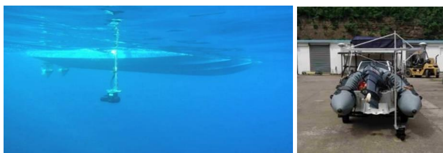
Fig. 14 – MBES Norbit iWBMSH integrated to Shom's deployable hydrographic system
