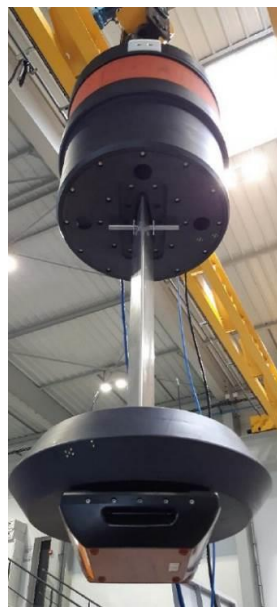
Fig. 28 - EM2040p MBES installed on its mount, deployable under the hull through the moonpool
