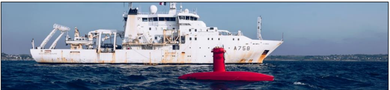
Fig. 43 - Experiment of USV DriX deployed from BHO Beautemps-Beaupré (Source: iXblue, 2020)
