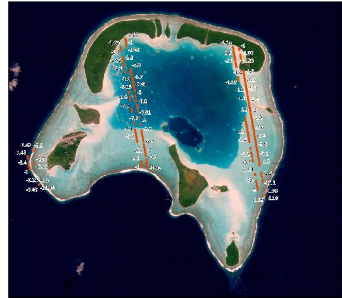
Data derived using EOMAP's Satellite Lidar Bathymetry toolbox and based on IceSAT-2 ATLAS data.
