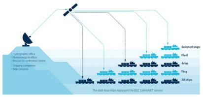
Figure 2 – Basic concept of the Inmarsat Enhanced Group Call system,
