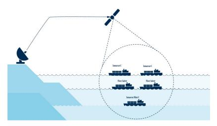
Figure 5 – SafetyNET service messages addressed to a circular area
