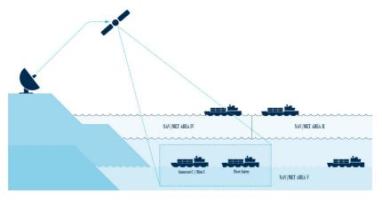
Figure 6 - SafetyNET service message addressing to a rectangular area
