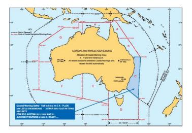
Figure 7 – SafetyNET services addressing to a coastal warning area
