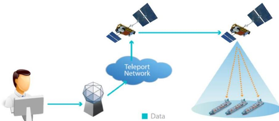
Figure 2 – Basic concept of the Iridium EGC system
