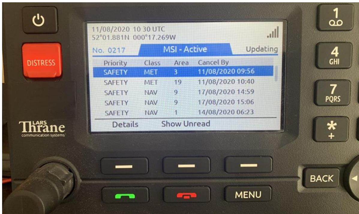
Figure 6 – Example of an Iridium SES Log Display
