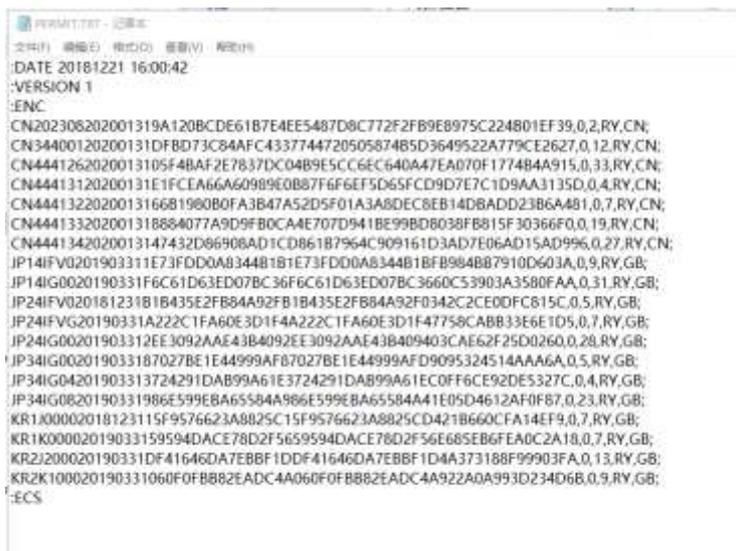
Fig. 3 Amendment of the Permit.txt file, the original Data Server ID was replaced by the Distributor ID (RY) and moved to the Comments section
