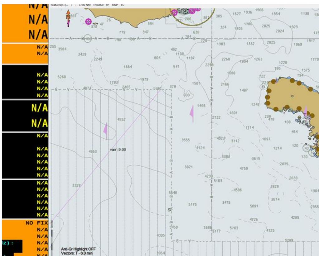
Figure: ECDIS unnecessarily displaying M\_NSYS symbology in-between different ENC products
