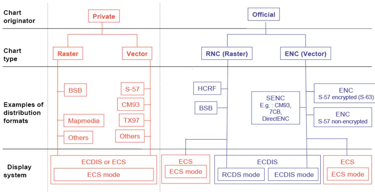
**Examples of Electronic Chart Formats. Many ECS systems are able to use ENC or RNC data, however even when using official charts they may not be used to fulfil ECDIS carriage requirements in accordance with SOLAS chapter V**
