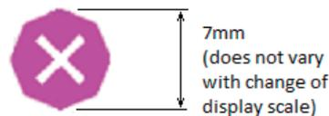
**Figure 6: Isolated danger (point) symbol in ECDIS**
