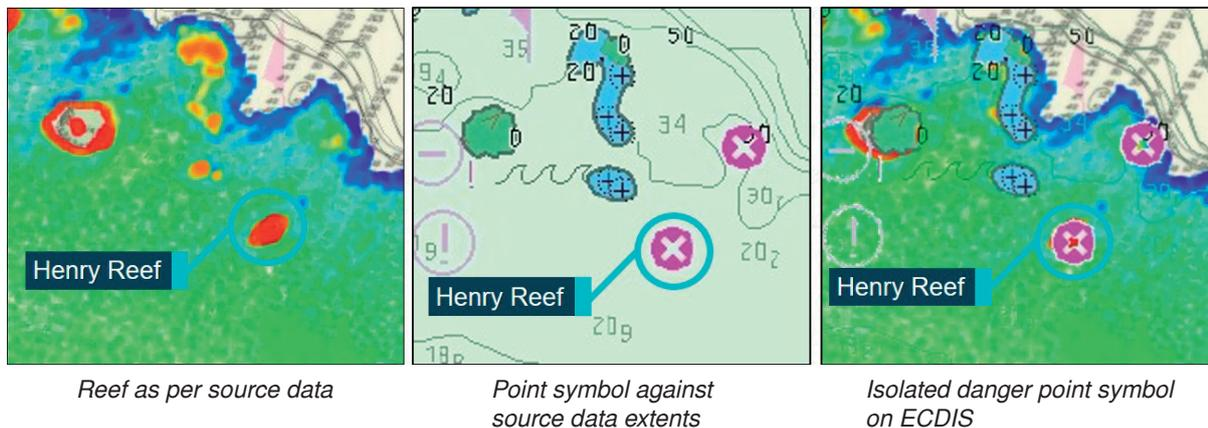
Figure 1: Comparison of small reef within source data at ENC compilation scale, point symbol depiction on ENC, and source data overlaid on ENC
