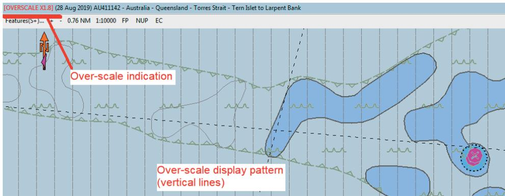
**Figure 7:** Over-scale indication and over-scale pattern on ECDIS
