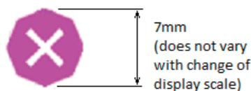
**Figure 6:** Isolated danger (point) symbol in ECDIS
