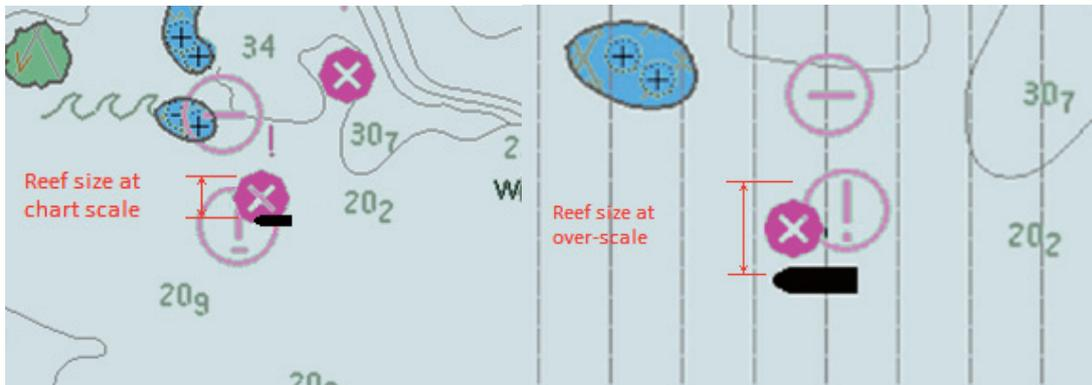
**Figure 8:** Over-scale indication and over-scale pattern on ECDIS
