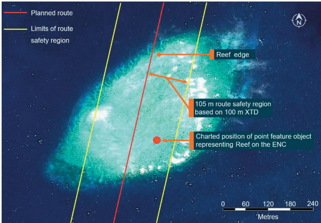
Figure 4: Planned route covers the position of the point symbol
