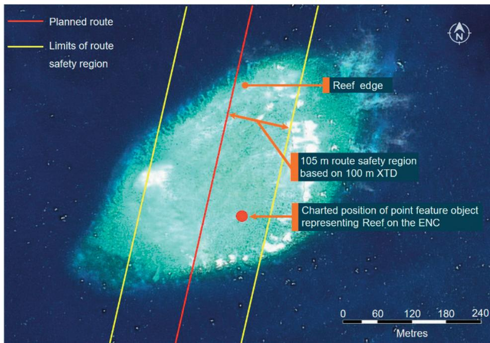
**Figure 4:** *Planned route covers the position of the point symbol<sup>2</sup>*
