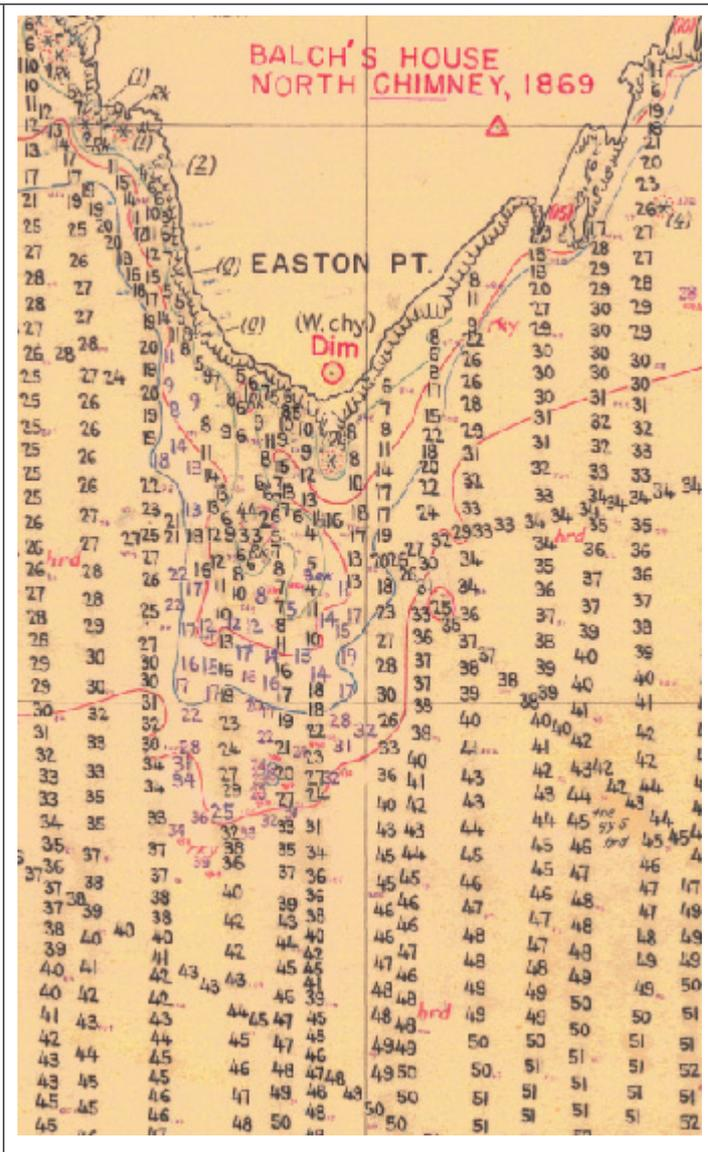
Figure 6-1 – Example: Systematic single beam survey from 1963
