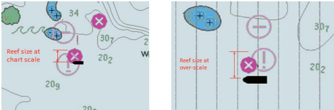
Figure 8: Over-scale indication and over-scale pattern on ECDIS
