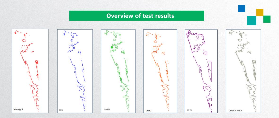
Generally speaking, we believe that the existing softwares can meet the requirements of HDENC production. At the same time, the depth contours auto-generated by different softwares are still different in some areas, and some of them need manual processing. However, the number of depth contours that need to be processed manually is small, which has a limited impact on the production efficiency of HDENC.
