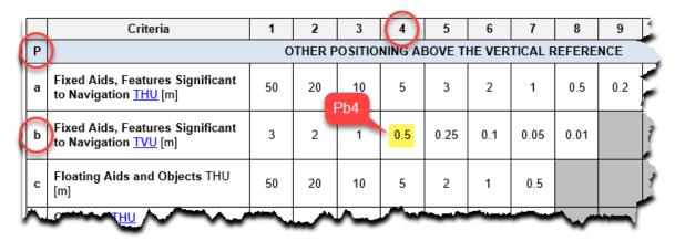
Figure A1 - Example: (Pb4) derivation of Fixed Aids, Features Significant to Navigation TVU = 0.5 m
