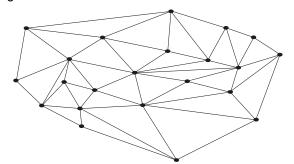
Figure 8-17 – An example coverage composed of TIN triangles
