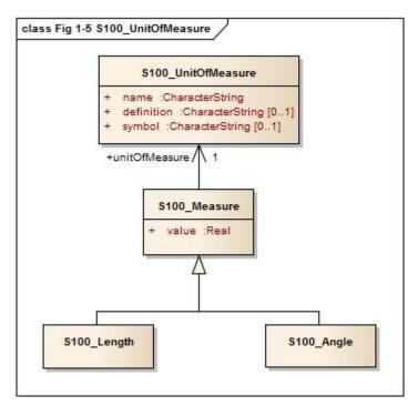
Figure 1-5 – S100\_UnitOfMeasure
