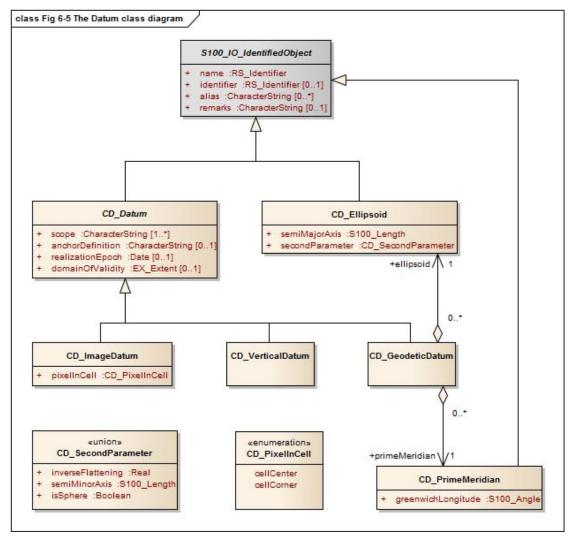
Figure 6-5 — The Datum class diagram
