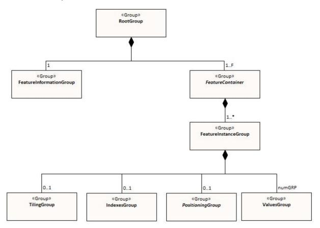
Figure 10c-7 - Basic structure of S-100 HDF5 file
