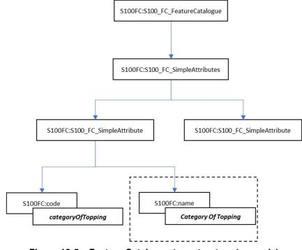
Figure 18-5 – Feature Catalogue tree structure (example)
