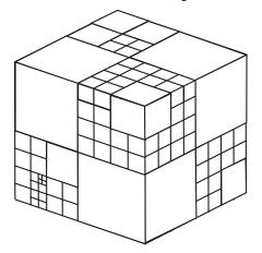
Figure 8-16 – A variable size cell grid in three dimensions
