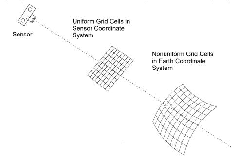
Figure 8-26 – Non uniform spacing of grid cells
