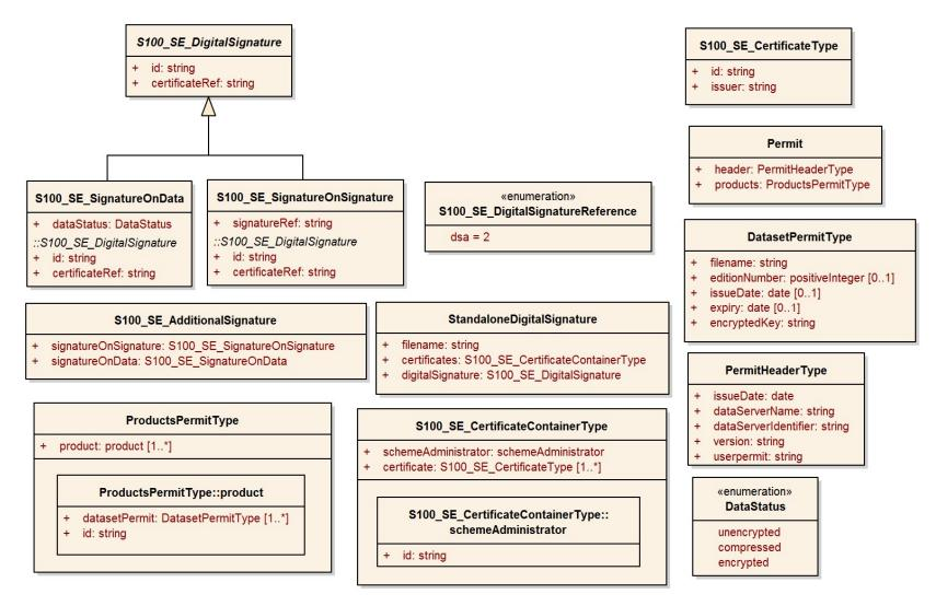
Figure 15-8 – Data protection – class details
