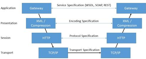
Figure 14-2 — Communication Stack
