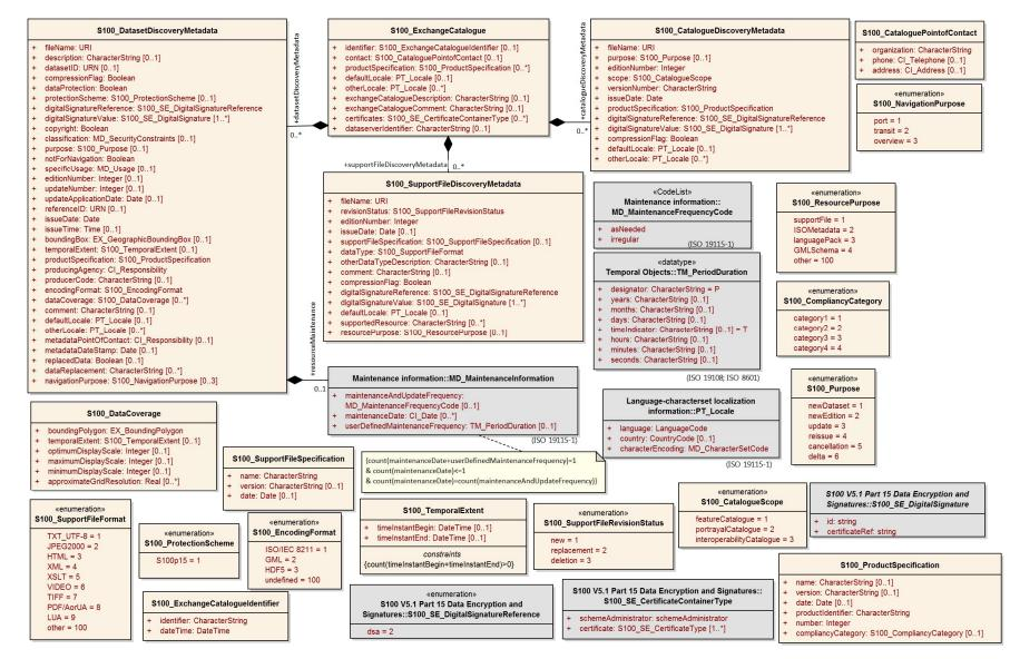
Figure 17-7 – S-100 Exchange Set Catalogue – class details
