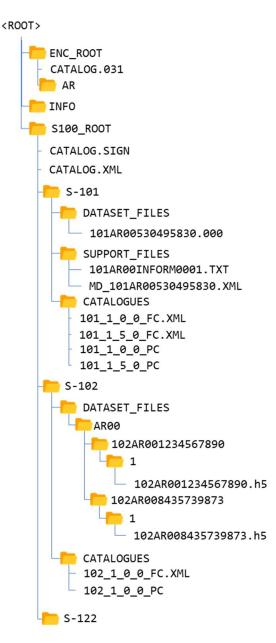
Figure 17-4 – Combined S-100 and S-57 Exchange Sets folder structure
