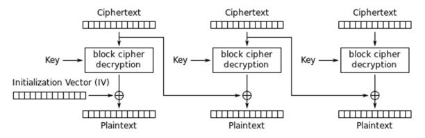
Figure 15-3 – Cipher Block Chaining (CBC) mode decryption (Source: Wikipedia)
