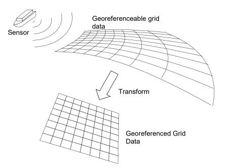
Figure 8-27 – Georectified data
