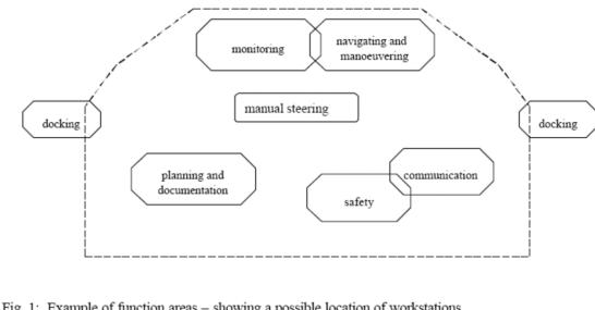
Fig. 1: Example of function areas - showing a possible location of workstations
