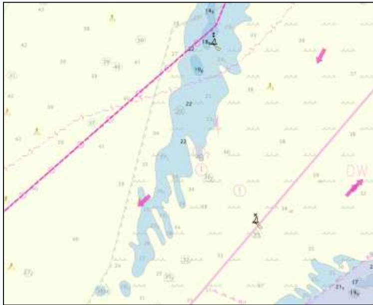
ECDIS with original ENC defaults to 30m contour
