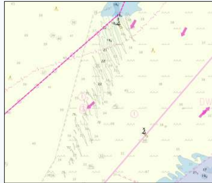
ECDIS with Band 6 high density ENC defaults to 22 m contour
