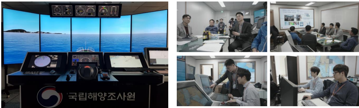
Fig. 3 S-100 Test Bed based on S-100 Navigational Simulator System
