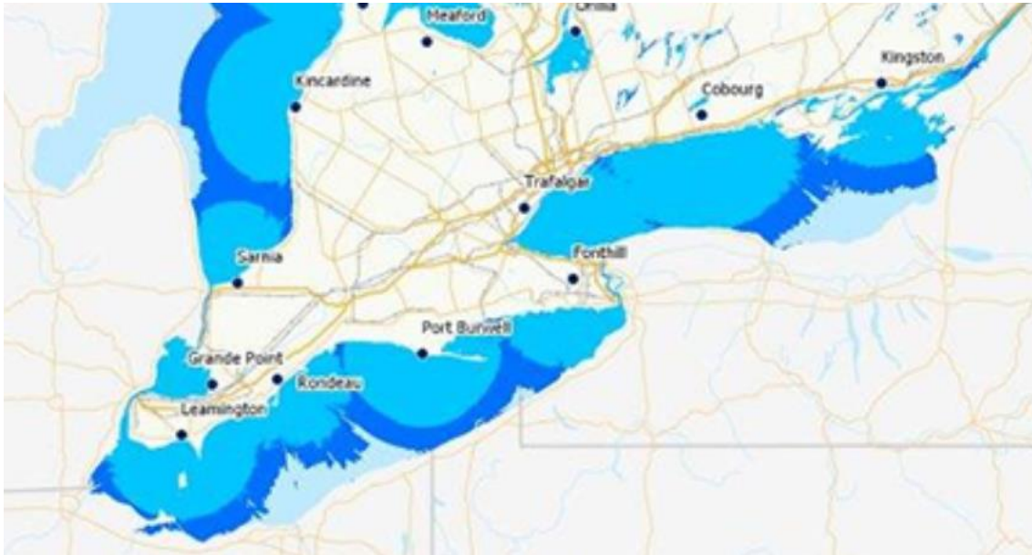
From CCG RAMN figure 4.5 Radio Coverage Prediction
