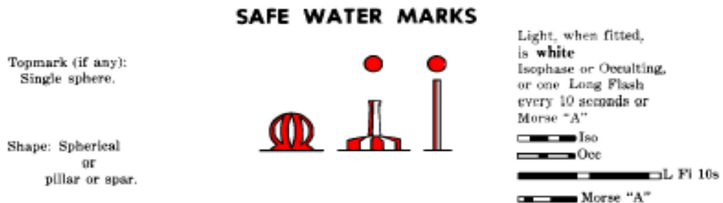
Figure 20-8 – IALA safe water beacons – Characteristics
