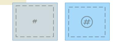
• S-101 has modified the centred symbol for foul ground this is a minor modification and consistent with S-4 (Principle 2)
