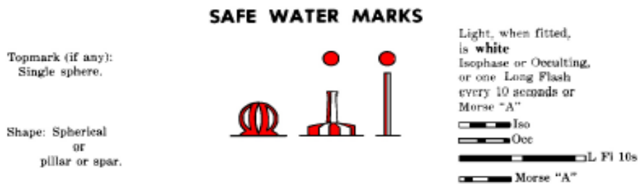
Figure 20-4 – IALA safe water buoys – Characteristics
