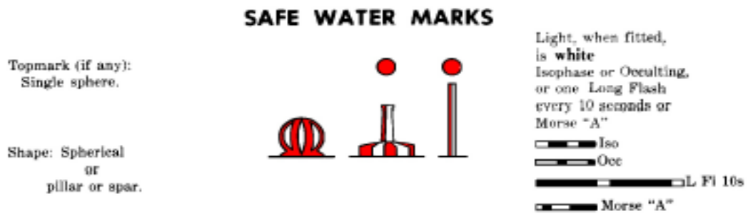
Figure 20-8 – IALA safe water beacons – Characteristics
