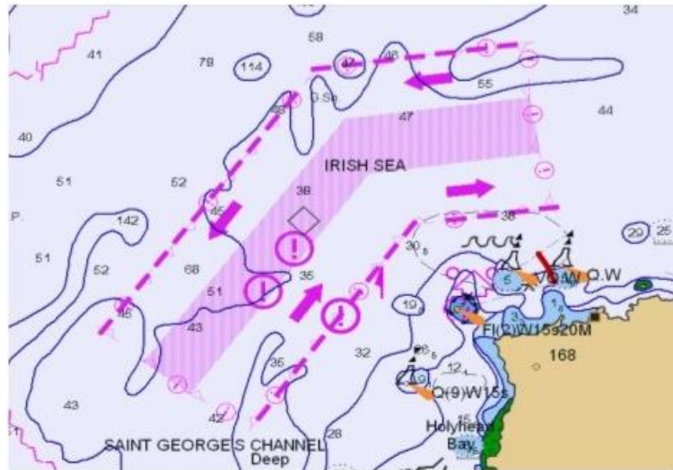
Figure 2-9 – Traffic Separation Scheme with appropriate masking
