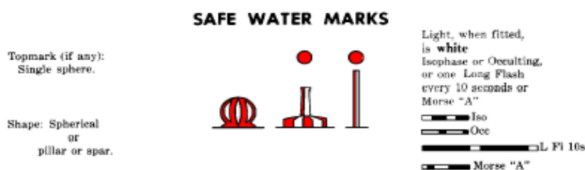
Figure 20.8 - IALA safe water beacons - Characteristics
