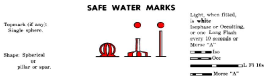
Figure 20.4 - IALA safe water buoys - Characteristics
