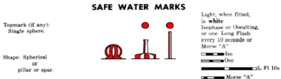
Figure 20.8 - IALA safe water beacons - Characteristics
