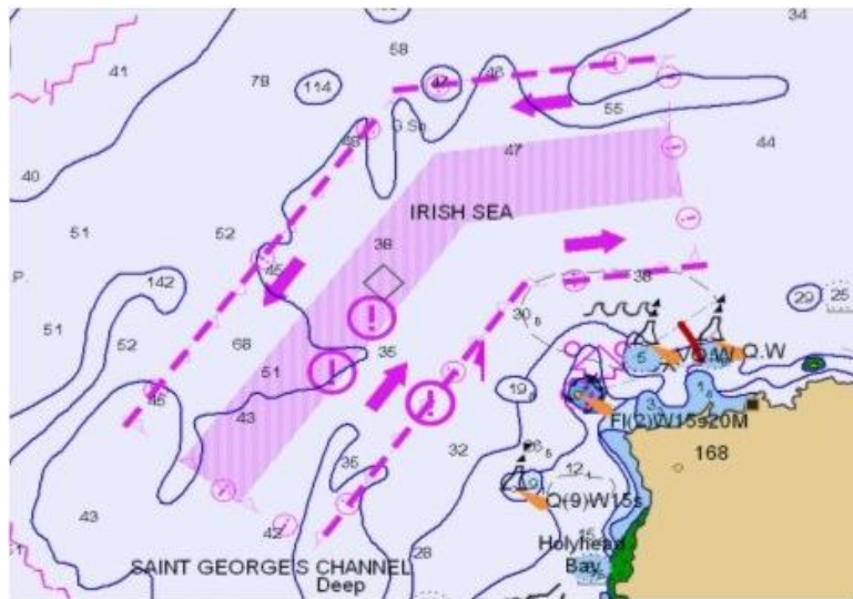
Figure 2.10 - Traffic Separation Scheme with appropriate masking
