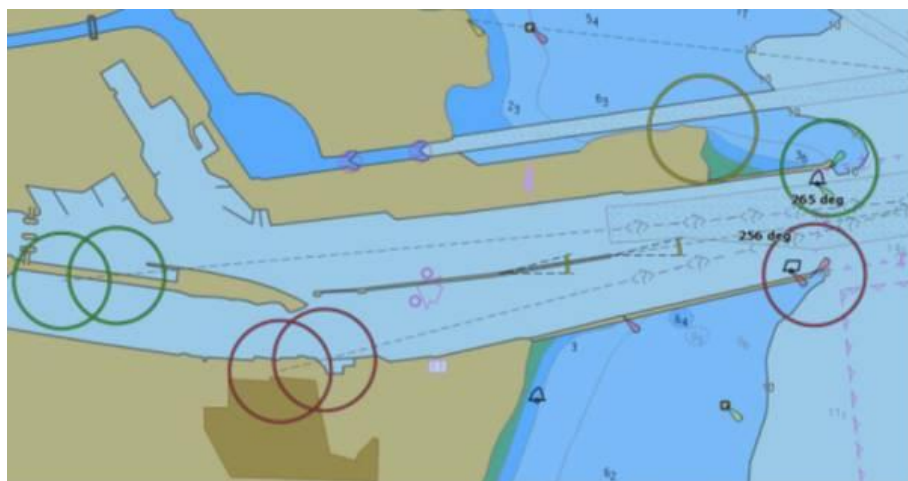
Figure 19.1 - Omnidirectional light display in ECDIS
