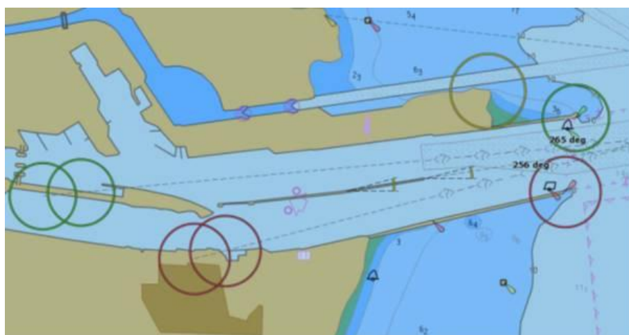
Figure 19.1 - Omnidirectional light display in ECDIS
