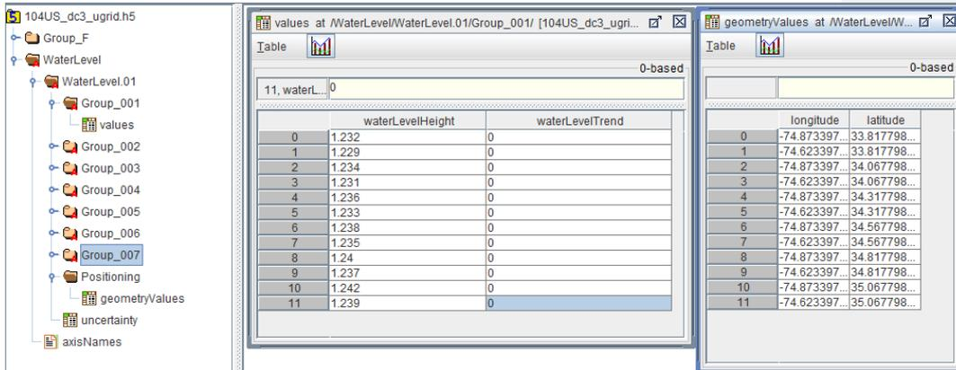
Figure E.13 – Sample HDF5 file (left panel) for ungeorectified gridded data. The middle panel shows the dataset ‘values’ and the right panel the dataset ‘geometryValues’
