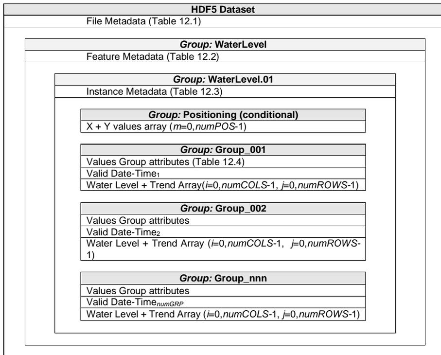
Figure 10.2 - Schematic of the S-104 HDF5 data product structure. The four parameters *numPOS*,
