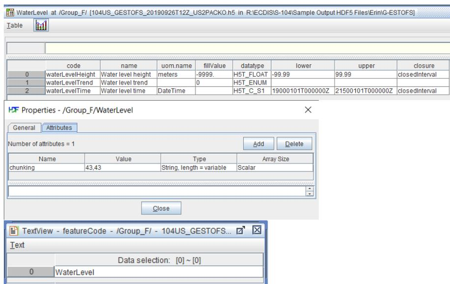
Figure E.2 - Group\_F includes the (top panel) compound dataset 'WaterLevel' and (bottom panel) the scalar dataset 'featureCode'. The dataset 'WaterLevel' (middle panel) contains the attribute 'chunking'. Values provided here for code (waterLevelHeight, waterLevelTrend, and waterLevelTime), uom.name (meters and DateTime), and fillValue (-9999. and 0) are required.
