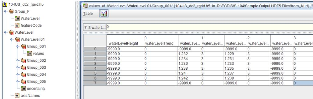
Figure E.10 – Sample HDF5 structure (left panel) and the dataset 'values' (right panel) for a two-dimensional array of regularly gridded data.
