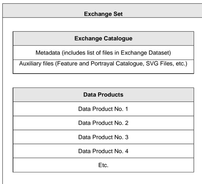
Figure 11.1 – Schematic diagram of the Exchange Set.
